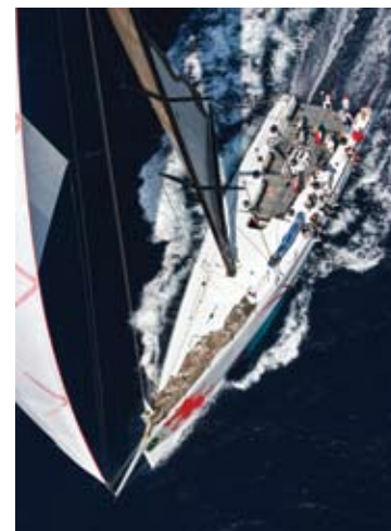
The 80ft maxi Beau Geste employs many innovative handling systems, including this gennaker system, which acts like a furling headsail, but the luff flies free from the stay. For more about Beau Geste see Boat of the Month, page 92
